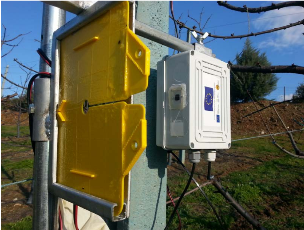
ReTIC: Real-time Trapping and Insect Counting The cases of Rhagoletis (Cherry fly) and D.Ciliatus (testing), and B.Zonata (testing)
